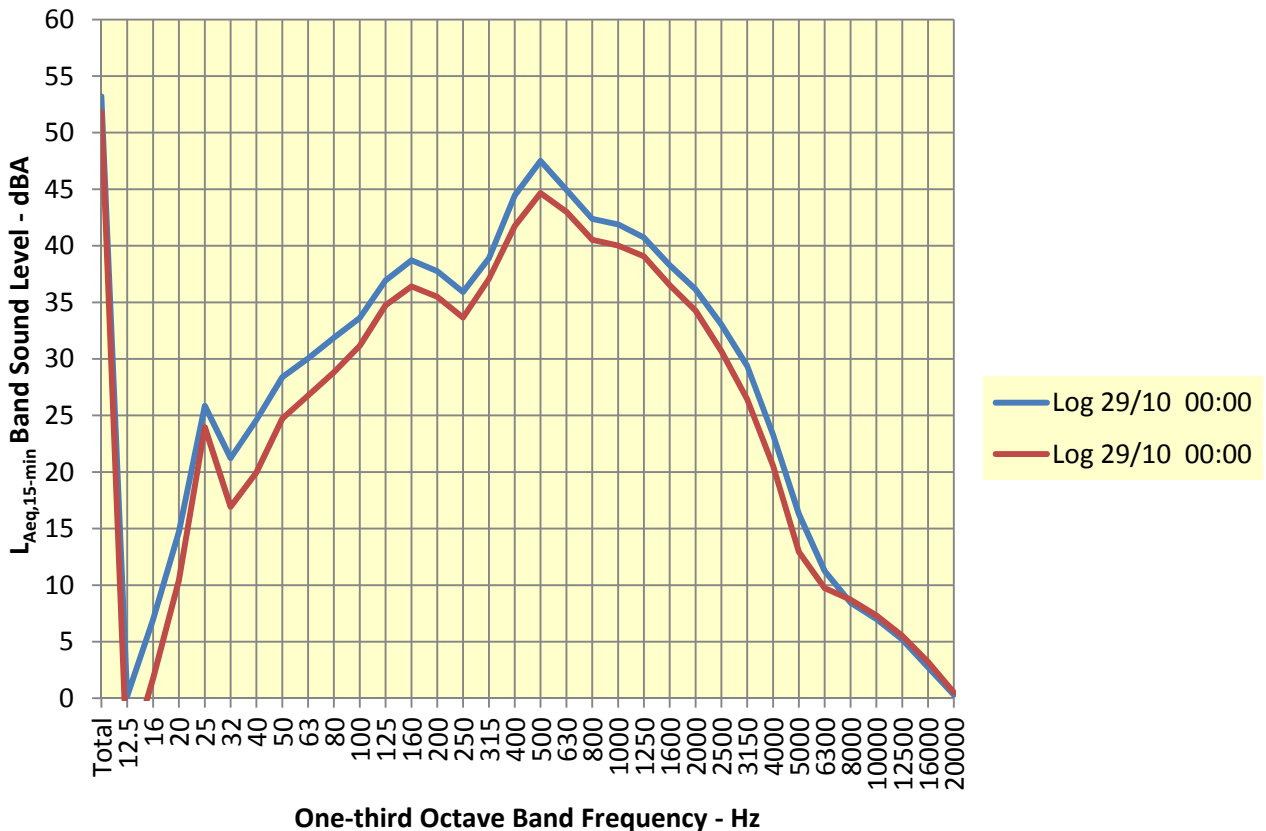
Figure F42: Boral Cement Berrima Annual Environmental Noise 2021 - Attended Monitoring Spectra: Location 20 L_{Aeq} & L_{A90}
