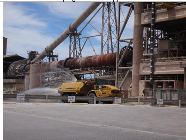
Photo 4- Water cart used for dust suppression
