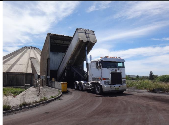
Photo 2- Truck dumping coal into hopper
