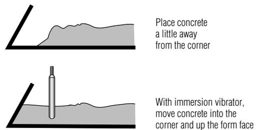
**Figure 5:** Compaction at stop ends and in inclined forms
