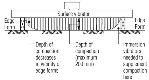
**Figure 8:** Degree of compaction varies across width when surface vibrators are used
