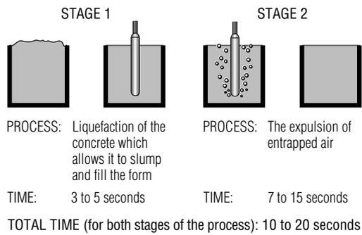
**Figure 1: The process of compaction**
