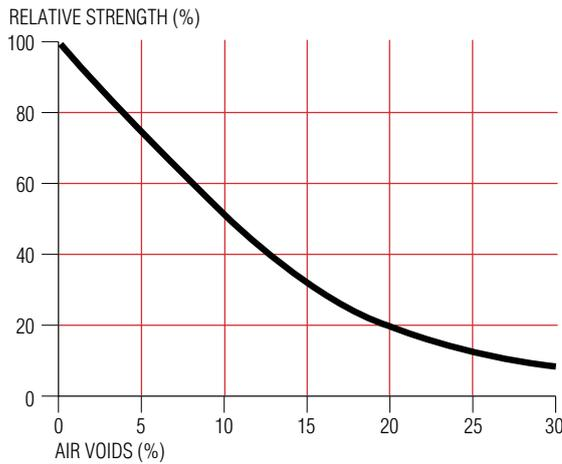
**Figure 2: Loss of strength through incomplete compaction**
