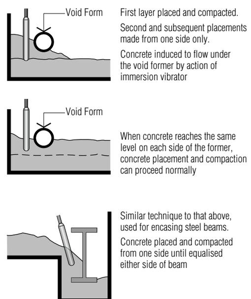
**Figure 6:** Compaction around void formers and encased members
