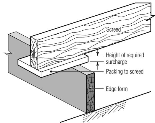
**Figure 9:** Method for providing a surcharge to the uncompacted concrete
