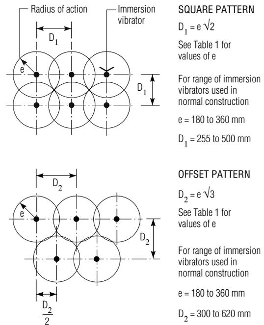
**Figure 4:** Alternative patterns for use of immersion vibrators
