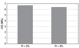
Note: Test method used - RMS T131 7 Day Accelerated (AC) UCS. (Samples @ 1 hour after mixing binder)
