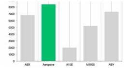
Fig5. Resilient Modulus (MPa)
