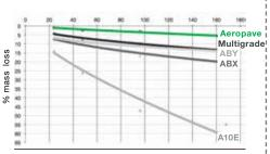
Fig2. Evaluation of Asphalt Fuel Resistance Soak Period (in Kerosene) [hours]
