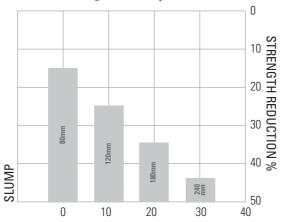
WATER ADDED: LITRES PER CUBIC METRE Concrete intially at 80mm Slump
